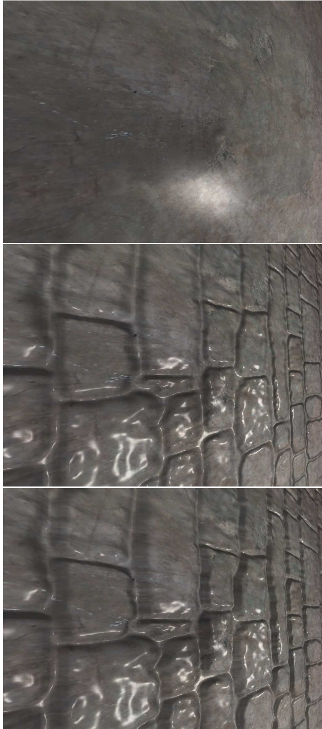
Figure 6.3: No added surface detail (top), normal mapping (middle), and normal mapping with parallax mapping (bottom)
