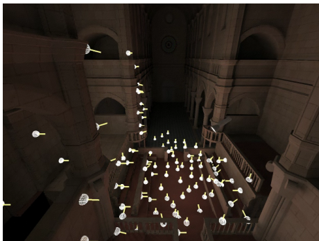
Figure 17: This figure shows the virtual point lights (VPLs) that have been created for the given spot light. They are evenly distributed in the viewing area of the point light.
