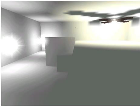
Figure 8: This image shows the same light map as in Figure 7, although this time a filter has been applied to smoothen the shadows.
