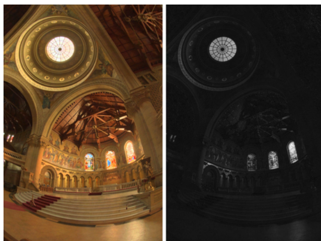
Figure 3. Memorial Church shown tone-mapped with Reinhard's global operator (left) along with the log-encoded ratio image needed for HDR recovery (right). 3
