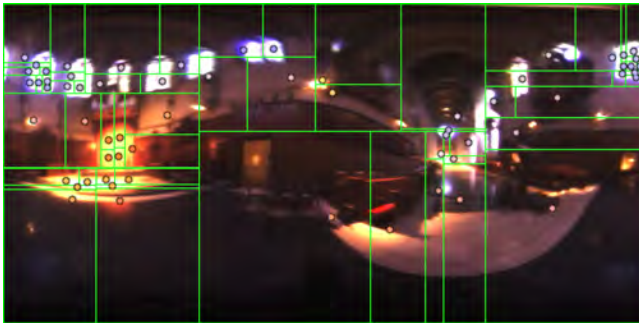
Figure 1: The Grace Cathedral light probe subdivided into 64 regions of equal light energy using the median cut algorithm. The small circles are the 64 light sources chosen as the energy centroids of each region; the lights are all approximately equal in energy.
