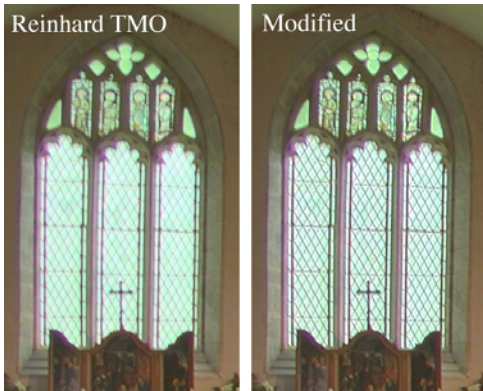
Figure 7. Reinhard's tone-mapping operator applied to the Dyrham Church image, before and after modification by the downsampled ratio image in our precorrection method. 3
