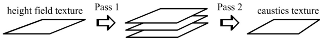
Fig. 4 The two-pass algorithm: the first pass reads the height field texture and generates multiple outputs; the second pass reads the result of the first pass and produces the final caustics map.
