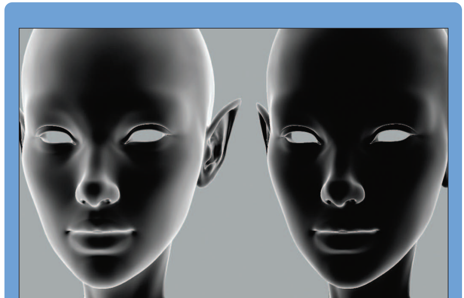
Figure 7: Dot products stored in SkinSilhouetteVec. On the left, (1 - (\mathbf{N} \cdot \mathbf{V})) ; on the right, (1 - (\mathbf{N} \cdot \mathbf{V}))^2 .
