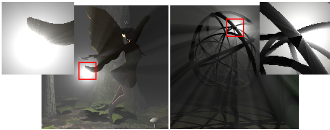
Figure 15: Epipolar regions may have poor \phi sampling, due to elongated voxels in this region. Angular aliasing occurs in regions with few occluded \phi samples. Noticeable artifacts above occur going from 0 \rightarrow 1 or 1 \rightarrow 2 \phi occlusions between adjacent epipolar planes.
