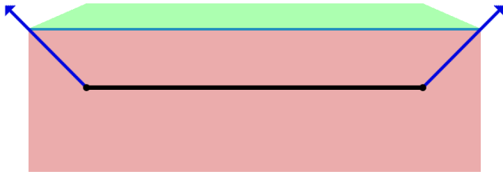
Figure 9-10: The house edge extends downward from the normal-offset points until the bottom of the inside edge is reached. This type of drawn edge covers much more area than other types.
