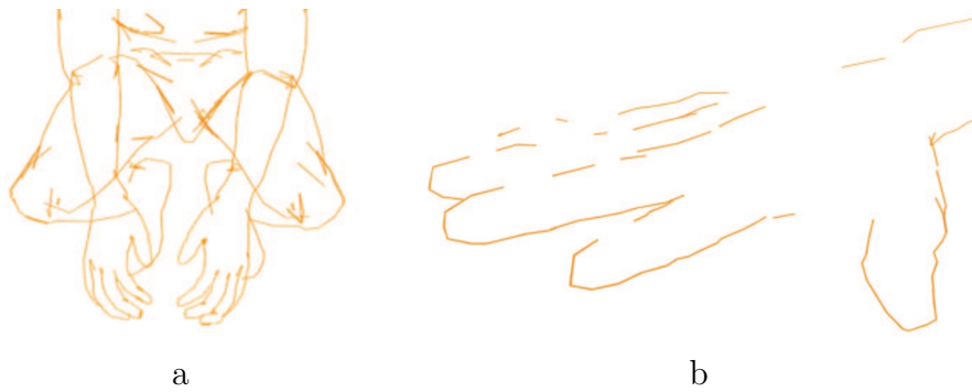
Figure 4.12: Problems of the Visibility Test a) Edges are only culled if they are completely invisible b) All edges that are not completely visible are culled leaving gaps
