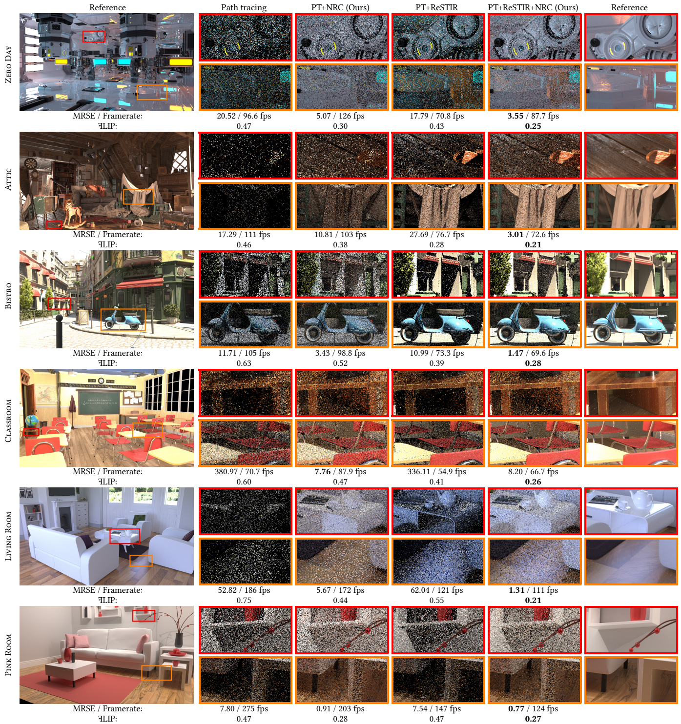
Fig. 10. We demonstrate the benefit of our neural radiance cache (NRC) in 1 spp real-time renderings with varied material and lighting complexity. From left to right: our baseline is unbiased path tracing with Russian roulette and next-event estimation driven by a light BVH [Moreau et al. 2019]. Then, we add spatiotemporal reservoir resampling (ReSTIR) [Bitterli et al. 2020] for low-variance direct and NRC for low-variance indirect illumination. Individually, these complementary techniques excel in their respective domains (e.g. ReSTIR in the directly lit BISTRO and NRC in the glossy ZERO DAY scene), but their combination unlocks the biggest improvement. Together, the three techniques reduce the mean relative squared error (MRSE) of path tracing by 1–2 orders of magnitude while incurring a comparatively little performance loss thanks to the drastic path shortening of NRC. In all scenes, the combined technique exceeds 60 frames per second at a resolution of 1920 \times 1080 . We also report the perceptually based \uparrow LIP metric that is more robust to outliers (“fireflies”).
