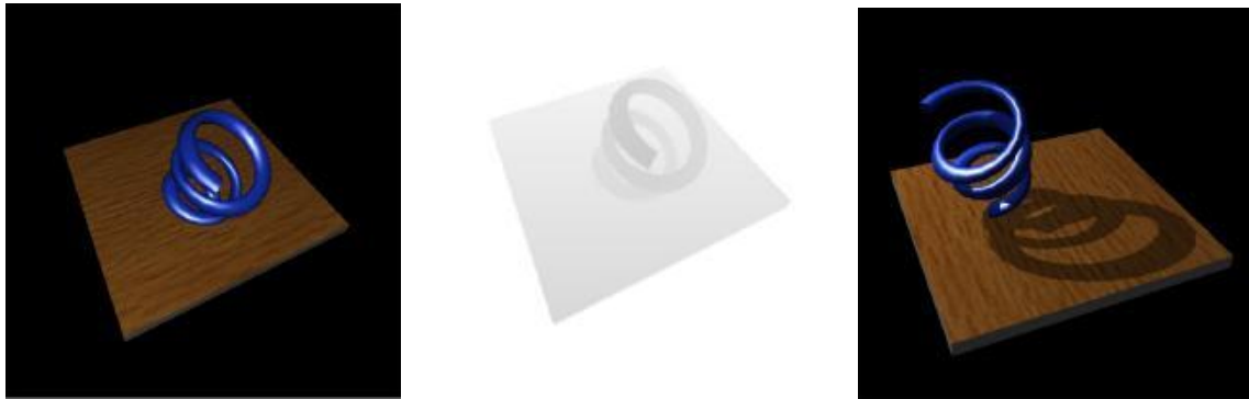
Figures 3.2.1-3.2.3: (Left) The scene as viewed from the light's point of view. (Center) A visualization of the shadow map, with darker pixels representing smaller depth values. (Right) The final image rendered from the camera's point of view.
