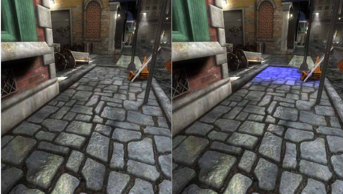
Figure 11. A complex scene with parallax occlusion mapping on the sidewalk and the brick wall. The strength of the blue tint in (b) denotes the decreasing level of detail (deepest blue being bump mapping and no blue displays full computation). Note the lack of visual artifacts and smooth transition due to the level-of-detail transition discernable in (a). The transition region is very small.
