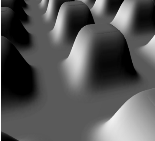
Figure 10. Smooth soft shadows and perspective-correct depth details generated with the parallax occlusion rendering algorithm
